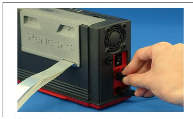
Figure 2.4 Connecting the host machine
